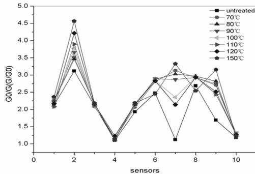
Figure 1. Relative conductivity of sensors on heat treated samples. The signals of the various samples obtained by sensors 1, 3, 4, 5 and 10 were very close. However, sensors 2, 7 and 9 were sensitive to changes because of its sensitivity to aldehydes, ketones, and heterocyclic compounds.
